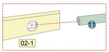
The protruding end of the part 11 needs to correspond to the hole of Section 02-1 when installed. Attach all screws for side 02-1 first and then attach side 02-2
